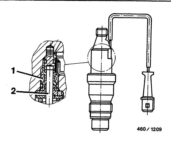
After cleaning a nozzle, the nozzle—and—holder assembly is to be reassembled with a 1 1 c o m p o—n e n t s p r e s e n t. If damaged components are established during disassembly, the nozzle—and—holder assembly is to be renewed.
